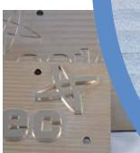
Our specially formulated system allows a clearance between the component parts to ensure that any crushing of the fluted board is kept to a minimum, delivering an effective and well-defined embossed result. If you're looking to elevate your packaging onto the premium platform, we can provide tooling that will enhance your graphics or simply lift the substrate with a contoured blind embossing. Wine boxes, beverage packs, confectionary
